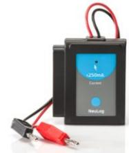
The shunt resistor is very high power (to protect it in high current) and very small resistance (in order not to affect the circuit conditions). The protection is up to 5 A.
