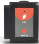
Once you have paired two RF communication modules to the same RF ID number (1 through 9) you can begin connecting NeuLog modules and sensors together. It may be easiest to imagine the RF communication modules as a long cable between the sensor and the USB module.
