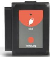
The USB module can be used as the power source for the sensors (instead of the battery module) and enables to start the off-line experiment at once for all of the connected sensors. This is for some complex experiments where more than one sensor has a trigger level and you want that the sensors' data will be synchronized.
