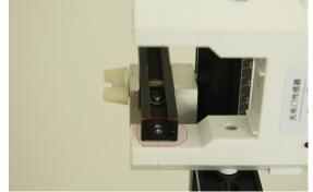
13. To find velocity with a photogate, measure the time the gate is blocked. Divide the marble's diameter by that time to find its instantaneous velocity.
