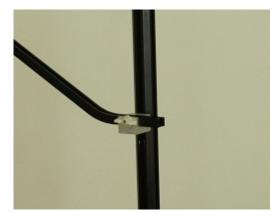
4. A consistent starting position can be indicated on the ramp using the included hardware. Decide which of the five starting holes you wish to use on the ramp and insert the Start Position Bolt into the starting hole on the horizontal ramp. This is held in place by using a metal wing nut which is threaded unto the machine screw from the underside of the ramp.
