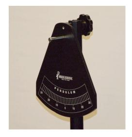
6. Align the Pendulum Face and Grid Board by using the string as a plumb bob. Face the stand, close one eye, and turn the pieces as needed so that the vertical lines are aligned with the string. Adjust the stand leveling bolts if necessary.
