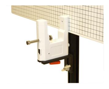
2. Grid Board (for selected experiments): Slide the small attachment bolt (ADO21c) down the channel in the workshop stand which is on the same side as the pendulum is mounted on. Insert the protruding bolt through the hole in the grid board, slide it up or down in the workshop stand channel to the desired height, and tighten firmly with the nylon wing nut (ADO21d).
