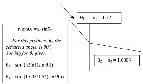
14. When all of the light bounces off the boundary of a material and none of the light escapes from the material, the light is totally reflected. Sketch the path that light takes in traveling through a large Plexiglas block when the light enters on one of the paths below.
